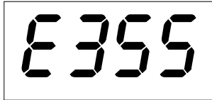
Figure 4. External Control Mode, 355 rpm
