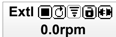
For External Current Signal 4-20mA
