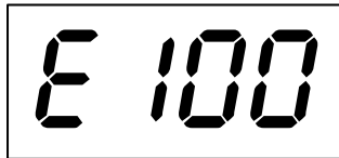
Figure 4. External Control Mode, 100 rpm.
