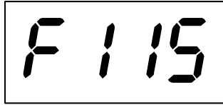
Figure 3. Easy Dispense Mode, 115 rpm
