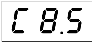
Figure 6. When flashing, pump is on Time Dispense Setup Mode
