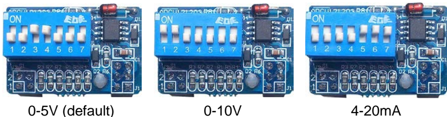
Figure 9. Analog Signal Control Board Setting
